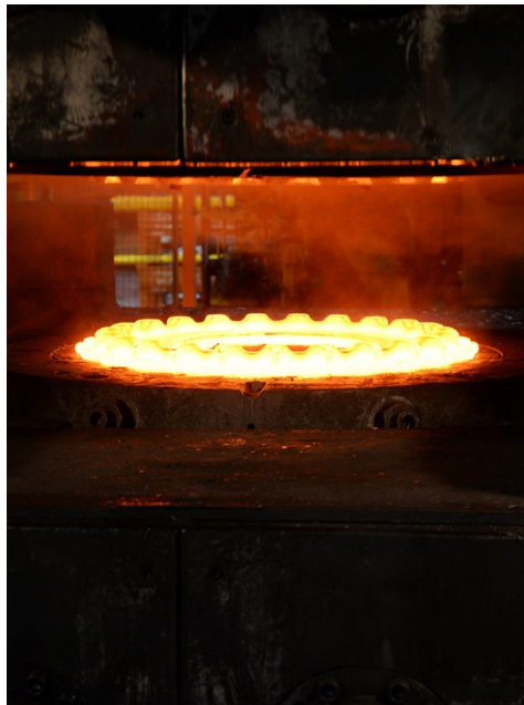
Forging a sprocket for mining excavators
